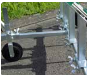
Adjustable spray angle/distance
