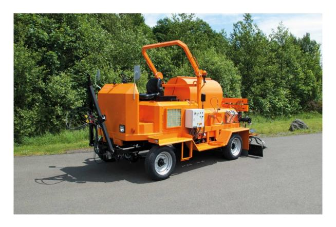
For spraying primer, bitumen emulsions and polymer-modified binding material.
